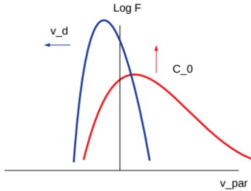
$$f_c(\mathbf{v}) = \frac{n_c}{\pi^{3/2} v_{th}^3} \exp\left(\frac{-(\mathbf{v} - \mathbf{v}_d \hat{v}_{\parallel})^2}{v_{th}^2}\right), \quad (1)$$
