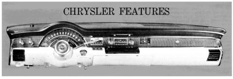
Chrysler's Instrument Panel not only is unmistakably premium-line in quality and appearance, it also reflects top-line planning in safety and convenience. The entire top and eyebrow of every Chrysler instrument panel is safety-padded and covered with nonglare vinyl. Instruments and controls are safety-recessed below the padded eyebrow and gauges are large and easy to read. The semi-circle speedometer, directly in front of the driver, has big, white numer-
