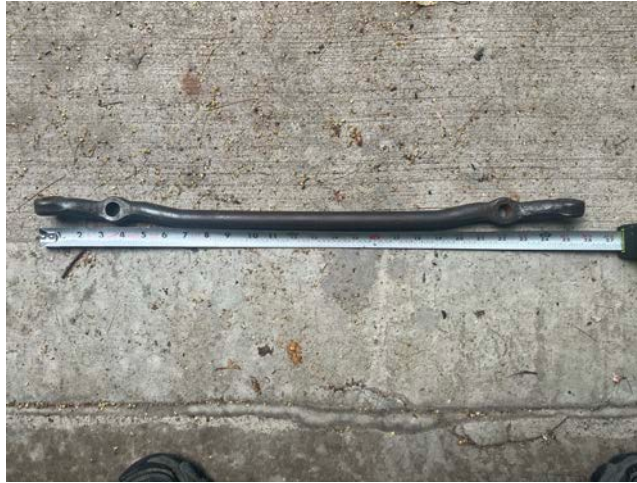
2 – Center link bars --- ~25.5" long – 1" bar (Tapered holes will have to be protected) (At least 1 Rods Possibly 2)
