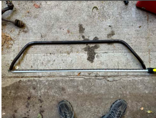
2 Sway bars --- ~45" -1" bar (Bent depth of 11") (At least 1 Rods Possibly 2)
