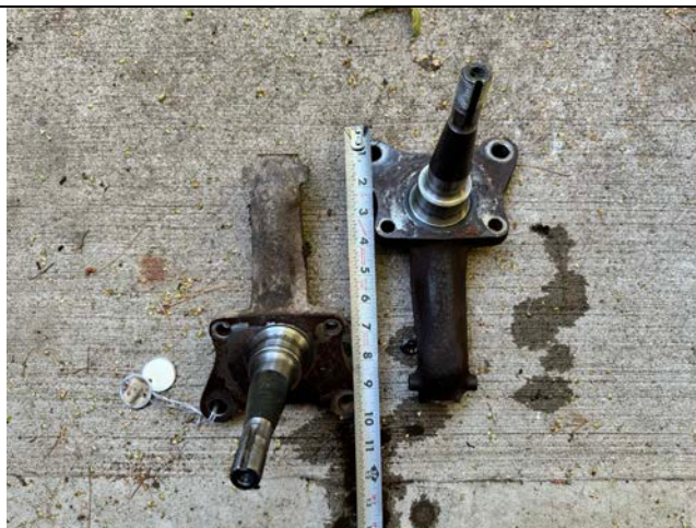
2 Steering knuckles with spindles that must be protected -- ~ 10" x 6" x 10"
