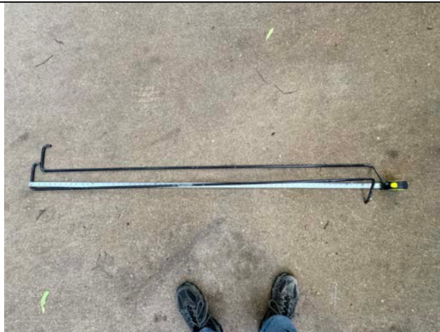
2 Torsion rods --- ~64" long – ½" rod (Bent depth of 11") One end of the rod will be booted for protection.
