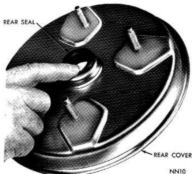
Fig. 6—Removing the Seal from the Rear Cover
